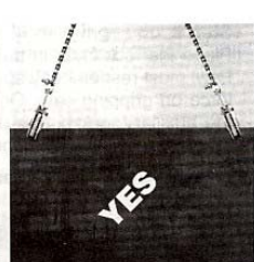
Photograph H. (Typical) Clamps in line with sling. (J and JA only)
