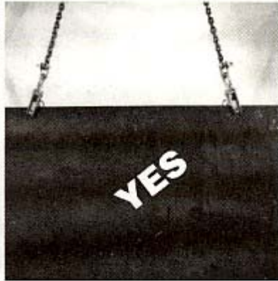
Photograph E (Typical) Clamps in line with sling.
