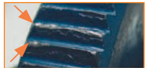
2 teeth damaged for 50%
