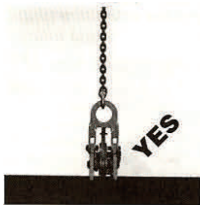
Photograph J Sling directly above and in line with the lifting shackle.
